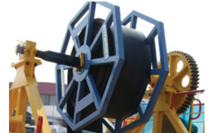
Fig. 2-5: Typical belt winder (with snub roll) set-up.
